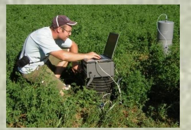
Greenhouse gas emission measurements with a photoacoustic sensor in an agricultural plot
