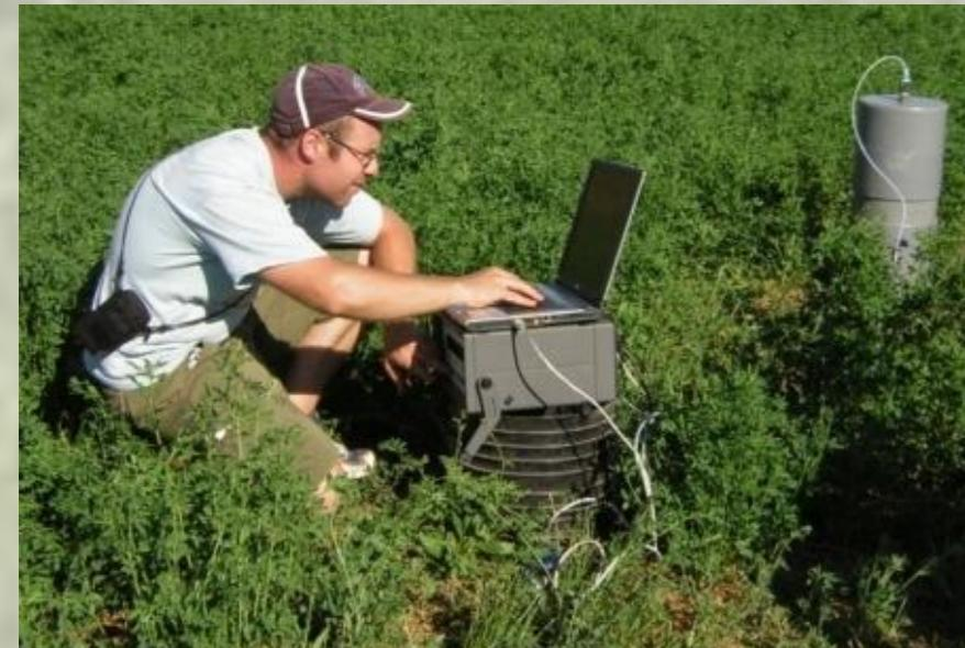
Greenhouse gas emission measurements in an agricultural plot with a photoacoustic gas-monitor
