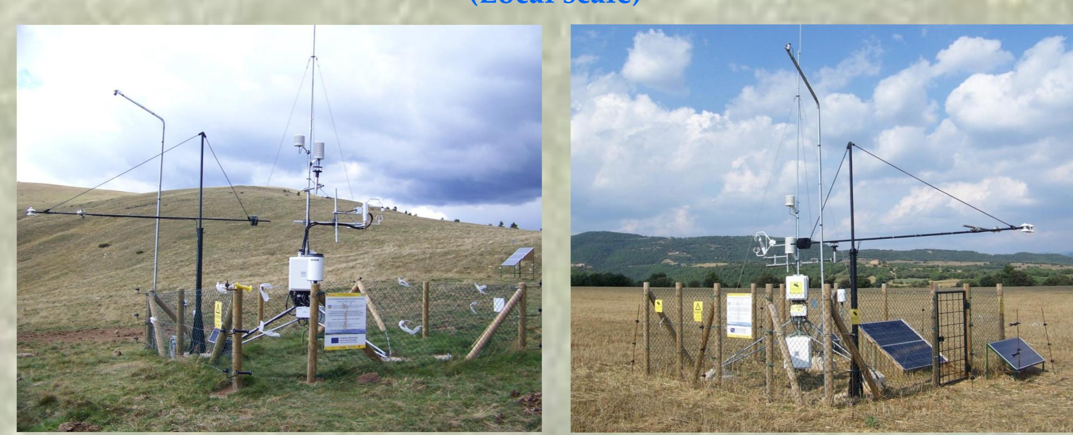
Three newly established micrometeorological stations (at 1000, 1300, 1900 m) for the monitoring of carbon, water and energy fluxes between the land and the atmosphere
