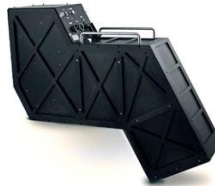
TASI (Thermal Airborne Spectrographic Imager ) 8 – 11.5 \mu\text{m} (32 bands mapping sensor)
